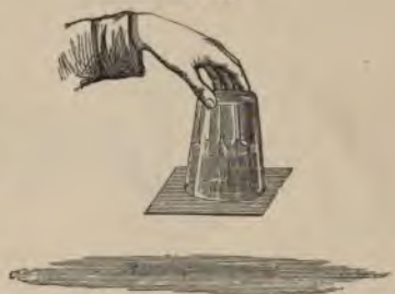
Inverted tumbler of water with card kept against it by atmospheric pressure.
